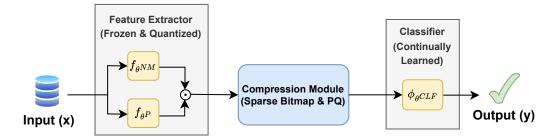
Figure 2: The system overview. LifeLearner consists of the frozen/quantized feature extractor, the continually learned classifier, and the compression module based on sparse bitmap and PQ. The compression module takes the feature extractor's outputs (activations) as inputs and compresses them to be saved as latent replay samples.
