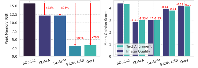
Figure 1: HierarchicalPrune achieves 79.5% memory reduction (left) while maintaining image quality. User study (right) demonstrates minimal quality drop (4.8-5.3%), contrary to the excessive degradation (11.1-52.2%) of prior methods.
